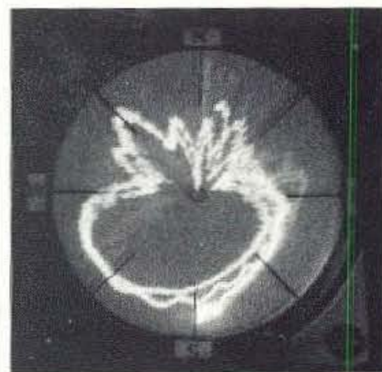
Photo B. This distant simplex signal is on the other side of a hill, so it has lots of multipath and airplane flutter. By viewing several overlaid sweeps with the NorthScope, it is clear that the most likely bearing is 235 degrees.
